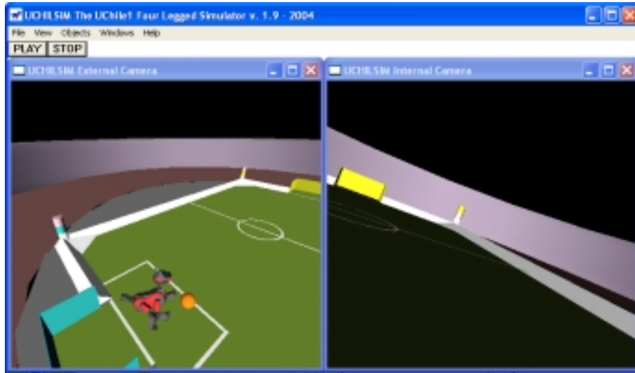
Fig. 6. Illustration of using the UCHILSIM simulator for learning to kick the ball. It can be seen in this case a curious behavior where the robot first pushes its body forwards and then kicks the ball with its right leg.
